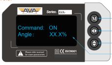
M button is used to enter and switch menus.
